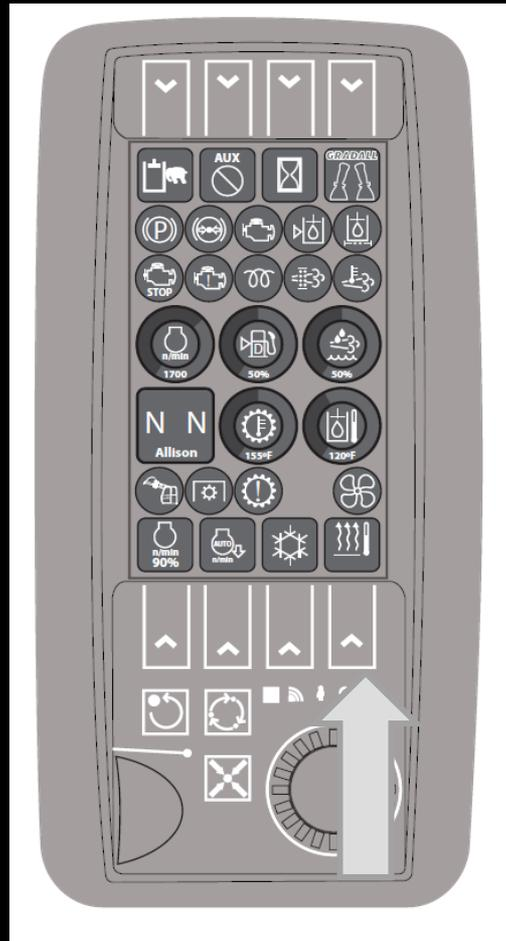
When the air conditioning is turned on you can not adjust the temperature, the air provided will be as cold as it can provide.
