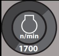
This is the engine RPM indicator. The actual rpm is displayed at the bottom of the icon.
