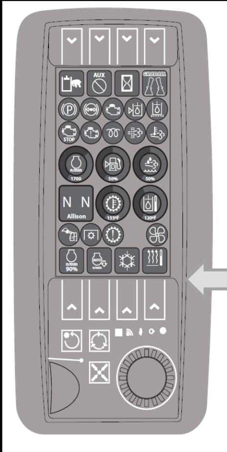
Across the bottom of the display are a row of buttons (5-8). These buttons activate the function/display of the bottom row of icons
