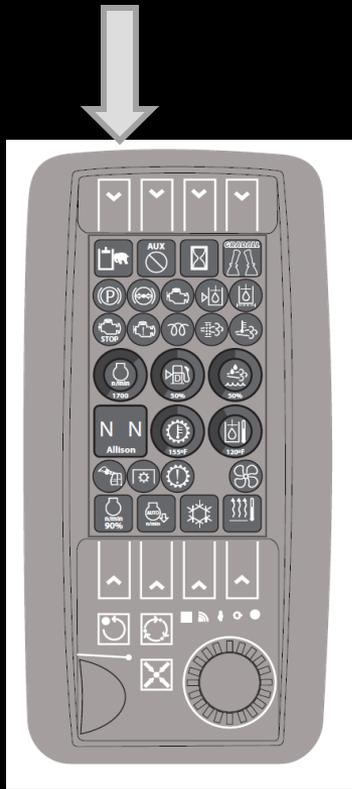
To turn the Fine Grade Mode on or off press the indicated button and the icon below the button will be enlarged turn the knob and the icon will change, when the desired function is displayed press the button again.
