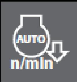
When the icon is **red** in color the auto idle is turned off when the icon is **green** the auto idle is turned on.
