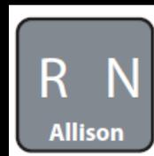
The transmission gear indicator on the monitor will show an “R” in the first position showing that reverse has been requested.
