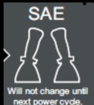
**SAE pattern:** Left joystick-extend and retract boom/swing the upper left and right; Right joystick-raise and lower boom/open and close the bucket.
