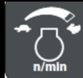
Press the indicated button to adjust the engine RPM. When the button is pressed the icon will enlarge in the middle of the display. Turn the dial to the right to increase rpm or to the left to decrease rpm.
