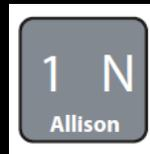
The transmission gear indicator on the monitor will show a “1” in the first position showing that 1<sup>st</sup> gear has been requested.
