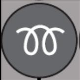
Icon 8 is the wait-to-start icon. When the icon is **yellow** the intake manifold heater is on. The engine will not start until the icon goes out.
