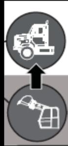
This is the remote/travel mode indicator. The icon of the truck cab will display in **yellow** until the required 70psi of air is available. The upper controls will not be active. As soon as the required air pressure is achieved the icon of the upper cab will appear in **green**; the upper controls will now be active.
