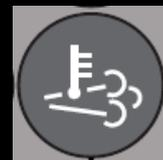
Icon 10 is the high exhaust temperature indicator. The icon turns **yellow** when the exhaust temperature is or is about to go above the normal operating temperature.
