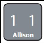
The engine RPM will drop and the transmission indicator will show a “1” in both positions indicating that the transmission has shifted in to 1<sup>st</sup> gear, the digging brake will release and the travel alarm will sound.
