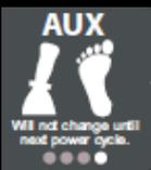
Auxiliary Hydraulics activated by pressing round button on front of the left joystick or the optional foot pedal.
