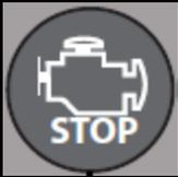
Icon 6 is the engine stop indicator. When a critical engine fault is detected the icon will turn **red** and an intermittent alarm will sound. Turn off the engine and contact service.
