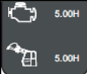
The total engine hours will be shown at the top of the icon and the operating hours from the upper will be shown at the bottom.
