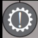
This is the check transmission indicator. It will light up in **yellow** to indicate that a problem has been detected in the transmission.
