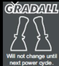
**Gradall pattern:** Left joystick-raise and lower boom/open and close the bucket; Right joystick-extend and retract the boom/swing upper left and right.
