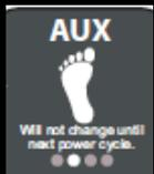
Auxiliary Hydraulics activated by pressing optional foot pedal.
