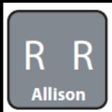
The engine RPM will drop and the transmission indicator will show an “R” in both positions indicating that the transmission has shifted into Reverse, the digging brake will release and the travel alarm will sound.
