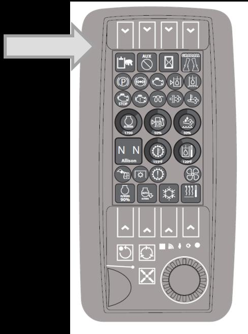
Across the top of the display are a row of buttons (1-4). These buttons activate the function/display of the top row of icons.
