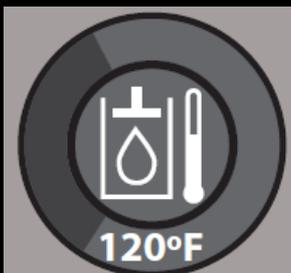
This is the hydraulic fluid temperature indicator. The actual hydraulic fluid temperature is displayed at the bottom of the icon.
