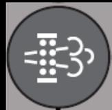
Icon 9 is the Diesel Particulate Filter Regeneration indicator. The icon flashes **yellow** when there is a need to regenerate the filter.
